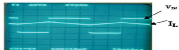
Fig.13 Inductor current I_L and V_{DS} Voltage
