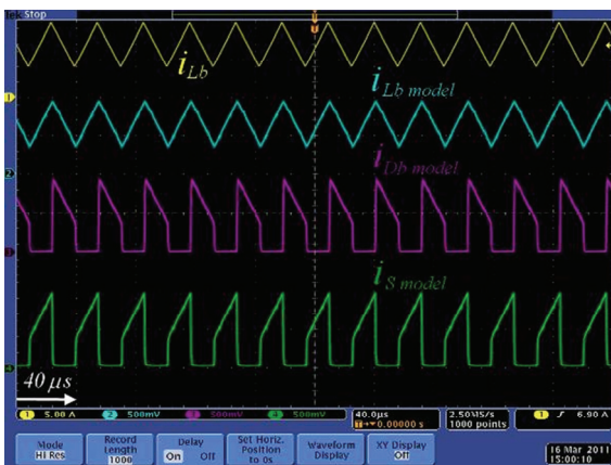
Fig. 20. Steady state waveforms: CH1 – i_{Lb} (experimental results), CH2 – i_{Lb\_model} (FPGA model results, 5 [A/div]), CH3 – i_{Db\_model} (FPGA model results, 5 [A/div]), CH4 – i_S\_model (FPGA model results, 5 [A/div])
