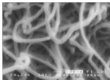
Fig. 1. A MWNTs original image taken by SEM
