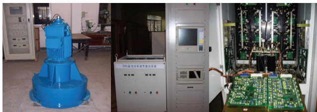
Figure.9 Experimental set with a DFIM , flywheel and back-to-back converters
