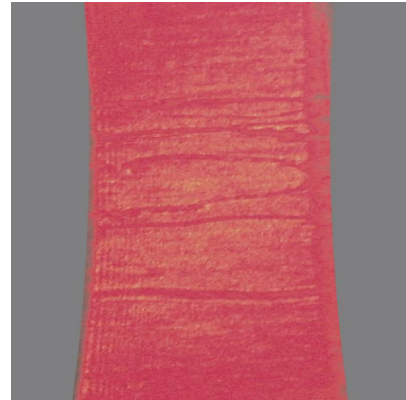
Fig.3 The picture of discharge gap at the applied voltage 1.2 kV and gap distance 0.4 mm.
