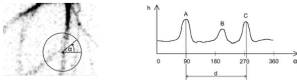
Fig.4. Histogram-based nodes and lines detection : weighted pixel intensity related to direction angle diagram and diagram calculation area
