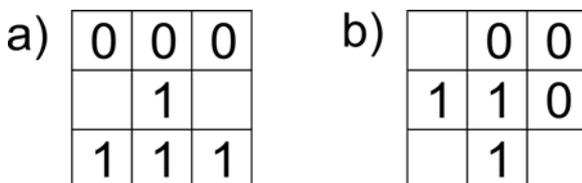
Fig.3. Structural elements for thinning operation
