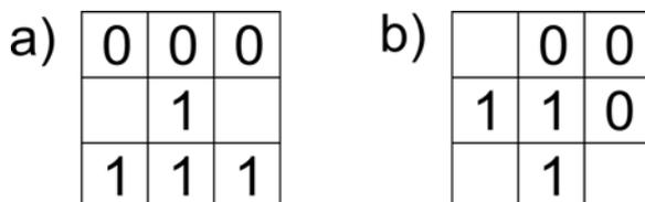
Fig.3. Structural elements for thinning operation
