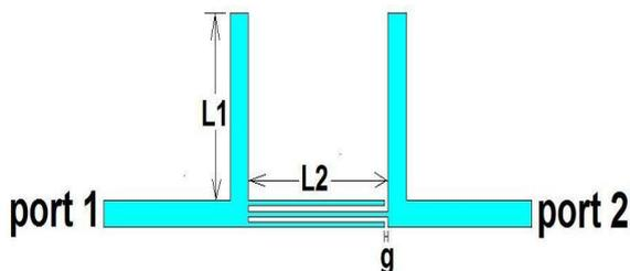
Fig.6. Layout of the proposed bandstop filter
