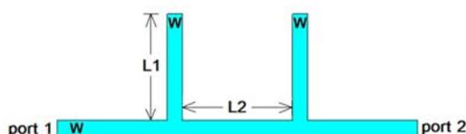
Fig.1. Layout of a conventional open stub bandstop filter
