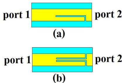
Fig.3. Configurations of spurline filters (a) single spurline (b) double spurlines
