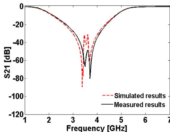
Fig.9. Comparison of simulated and measured transmission coefficients ( $S_{21}$ ) for the proposed filter
