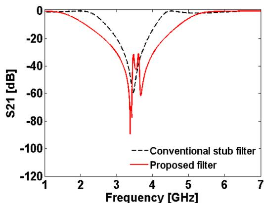
Fig.7. Comparison of simulated transmission coefficients ( $S_{21}$ ) for the conventional open stub filter and the proposed filter
