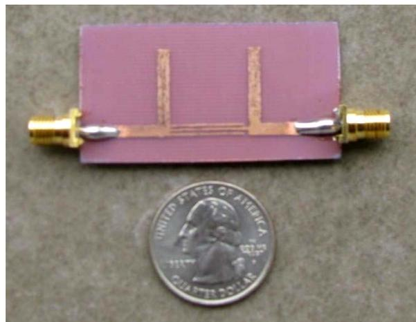
Fig.8. The photograph of the proposed bandstop filter
