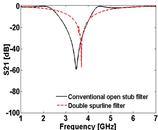
Fig.5. Comparison of simulated transmission coefficients ( $S_{21}$ ) for double spurline filter and conventional open stub filter
