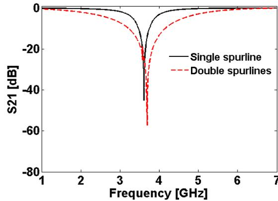
Fig.4. Comparison of simulated transmission coefficients ( $S_{21}$ ) for single spurline filter and double spurline filter
