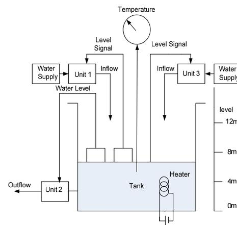
Fig. 1 Water Level and Temperature Control System
