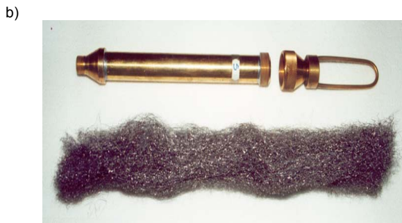
Fig. 2. Superconducting matrix separator for HGMS: a) scheme of the separator, b) matrix of the separator and their filling
