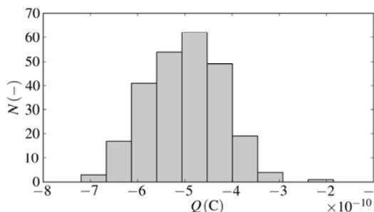
Fig. 5. Distribution of charges of the PVC particles
