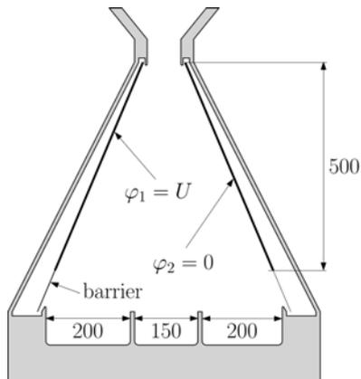
Fig. 2. Arrangement of the investigated device (dimensions in mm)
