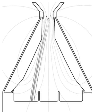
Fig. 9. Trajectories of the PET particles
