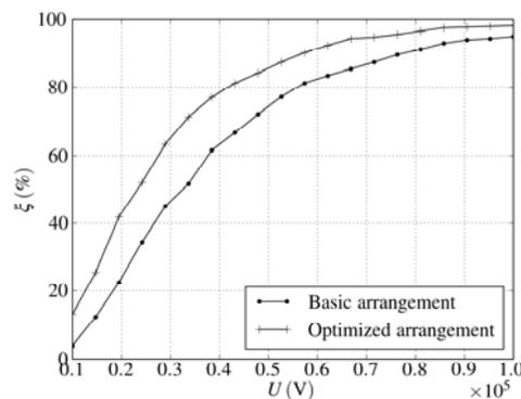
Fig. 10. Efficiency of the separation process as a function of voltage for the basic and optimized arrangements
