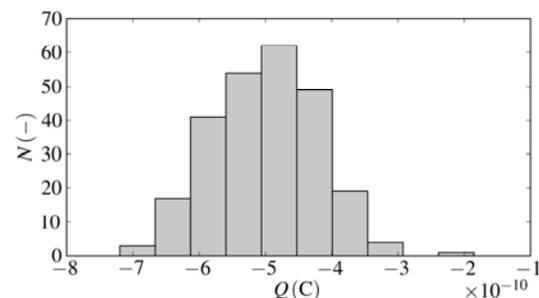
Fig. 5. Distribution of charges of the PVC particles
