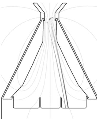
Fig. 8. Trajectories of the PVC particles
