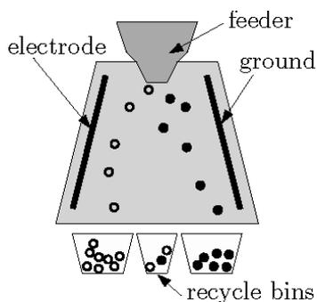
Fig. 1. Typical separator of plastic particles based on the triboelectric effect
