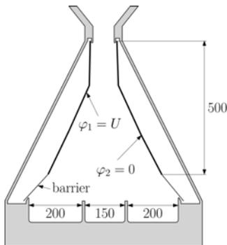
Fig. 7. Optimized arrangement of the electrodes
