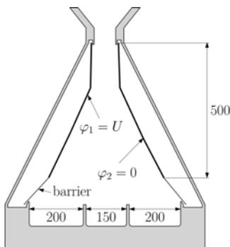
Fig. 7. Optimized arrangement of the electrodes
