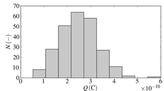
Fig. 4. Distribution of charges of the PET particles
