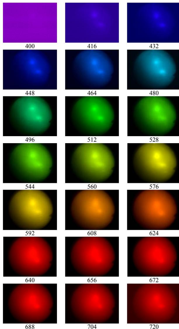
Fig. 2. A series of multispectral images obtained for skin tissue with centrally located cancer region. The numbers below figure are central wavelengths of transmitted bands expressed in nanometers
