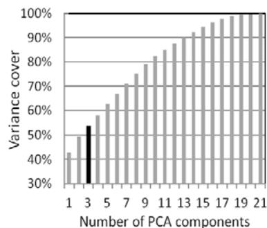
Fig. 4. The covariance cover as the function of the number of PCA attributes applied to the same image processing as that seen in figure 2. The case of three spectral attributes is marked (compare with figure 3)
