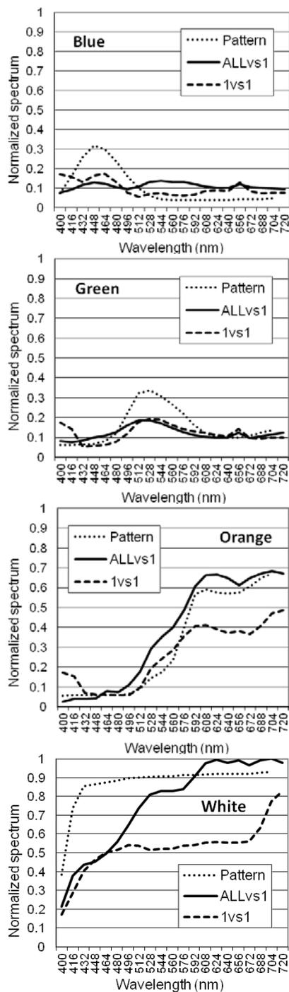
Fig. 3. Measured, during the training procedure, the normalized spectra of the selected colors; for blue, green, orange, and the white colors using the '1vs1' and the 'ALLvs1' methods. The registered spectra are compared with a standardized, ideal pattern. The 21 values of wavelengths, at abscissa, define the central positions of spectral windows used in experiments
