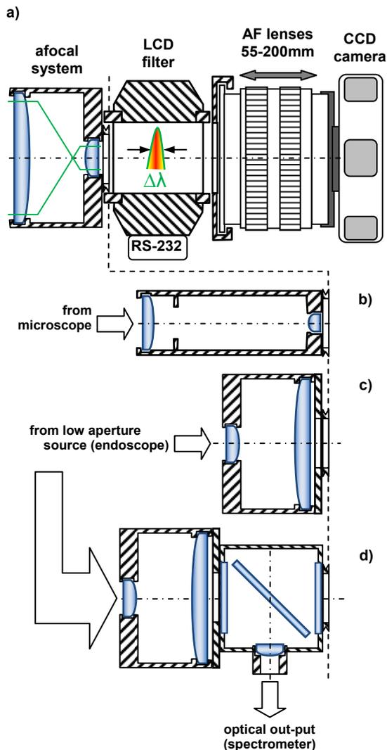
Fig. 1. Construction details of the opto-mechanical system (a), the afocal lenses can be substituted directly by a microscope ocular (b), by reversing the afocal lenses it can be coupled with a low-aperture device (c), or (for all above cases) the system can be modified by a beam-splitter to provide a fraction of signal to the optical spectrometer (d)
