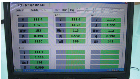
Fig.7. Monitoring and management interface of wireless automatic meter reading system
