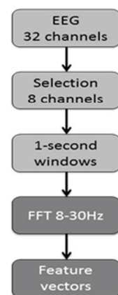
Fig. 2. The scheme of feature extraction
