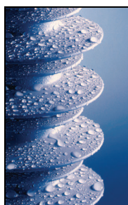
Fig. 1. The hydrophobic properties of the surface of the polymeric insulator [1]
