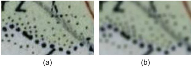
Fig. 2. Fragment of image before (a) and after (b) low-pass filtering.
