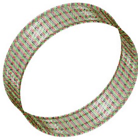
Fig.2. The whole stator coils
