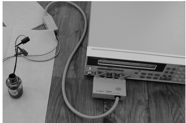
Fig. 5. Quick operative permeability measurement arrangement with the RLC bridge
