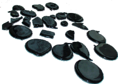
Fig.6. The safe vitrificate formed into ceramic tiles.
