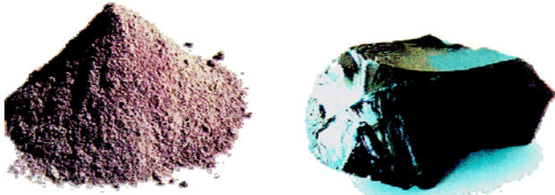
Fig.5. Solid waste containing heavy metals with organic residues compared to non-leachable vitrificate in plasma furnace
