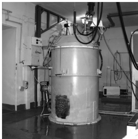
Fig.3. The plasma arc furnace.
