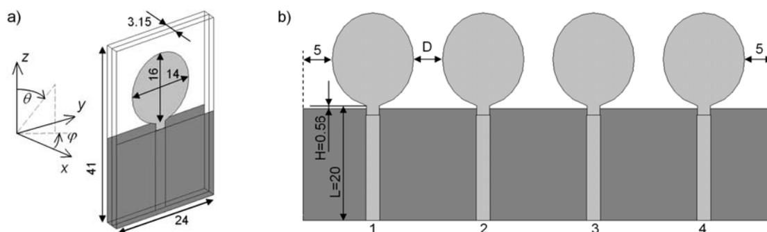
Fig.1. The structure of a basic single UWB antenna (a) and the example of a 4-element UWB antenna array (b) (dimensions in mm)
