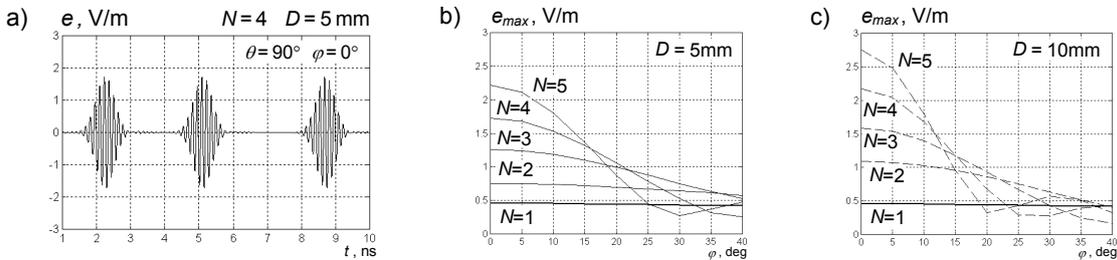
Fig.4. Pulse shapes of an electric field radiated by a 4-element UWB antenna array and amplitudes of pulses radiated by a 4-element array in x-y plane for different directions (b,c)
