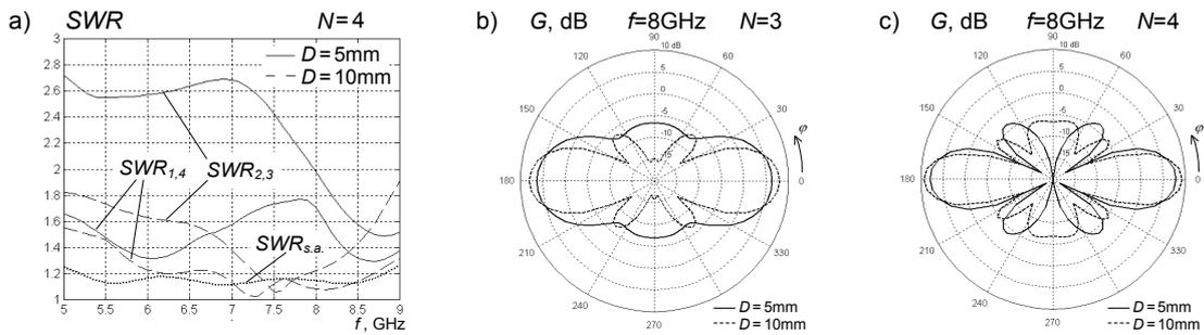
Fig.2. SWR (a) and radiation patterns (b,c) of selected models of antennas
