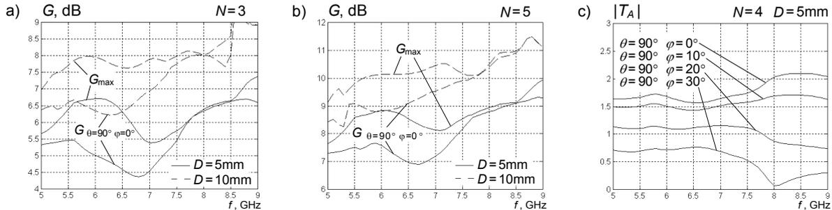
Fig.3. Antenna gain for different arrays (a,b) and modules of a 4-element antenna array transmittance for different directions
