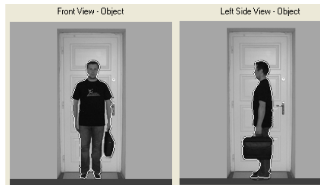
Fig. 6. Images with a marked border of an object detected inside a mantrap using the operation of subtraction, source: own material
