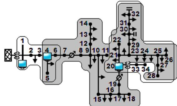
Fig. 3. Coverage area for optimal PQMs placed at buses 1, 4 and 20 for the IEEE 34-node system.
