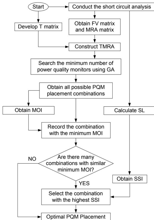
Fig. 2. The overall optimization flowchart
