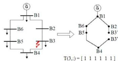
Fig. 1. Example of row 3 in T matrix for different system topologies
