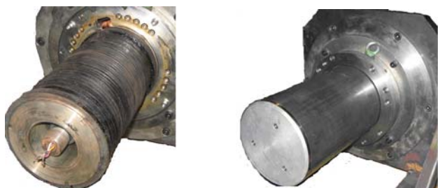
a) The stator of induction heater b) Induction heater Fig. 11 Prototype of the induction heater.
