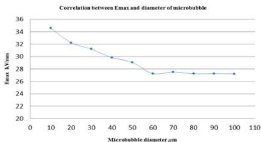
Fig. 8. Correlation between Emax and diameters of microbubbles
