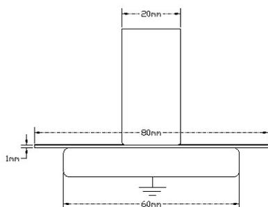
Fig. 2. Simulation model of surface discharge in oil-paper insulation
