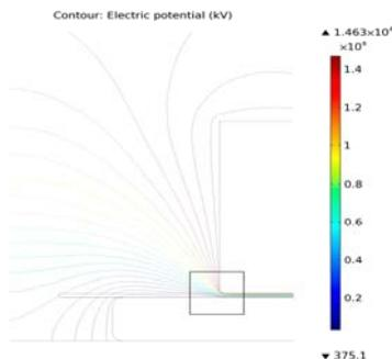
Fig. 3. Equipotential lines of the surface discharge model (at the phase of 90 deg)
