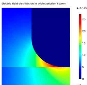
Fig. 4. Electric field distribution in triple junction region
