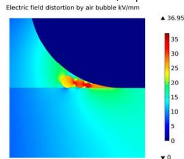
Fig. 7. Electric field distortion by air bubbles
