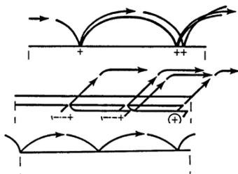
Fig. 1. Electron paths along surface of insulator according to gas discharge theories [12]
