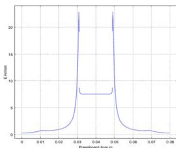
Fig. 5. Electric stress distribution along the insulation pressboard
