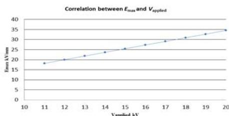
Fig. 6. Correlation between  $E_{max}$  and  $V_{applied}$
