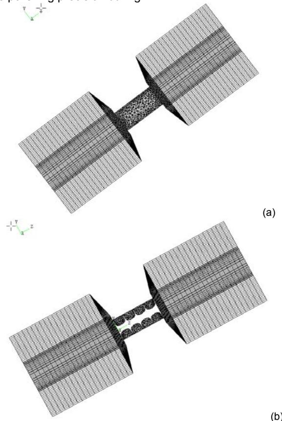
Fig. 4. CFD modeling diagram of the abrasive medium (a) without a helical passageway. (b) with a helical passageway.
