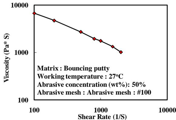
Fig. 1. The curve diagram of viscosity relative with shear rates
