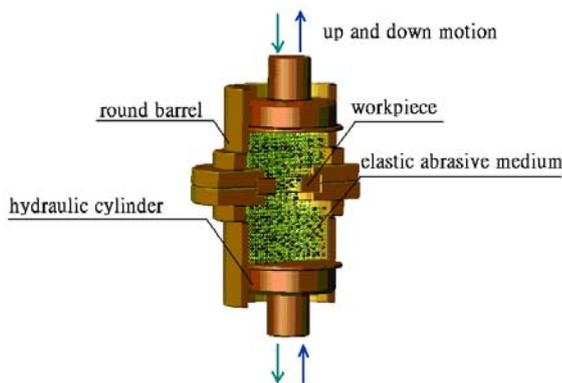
Fig.2. Diagram of machining process in AFM
