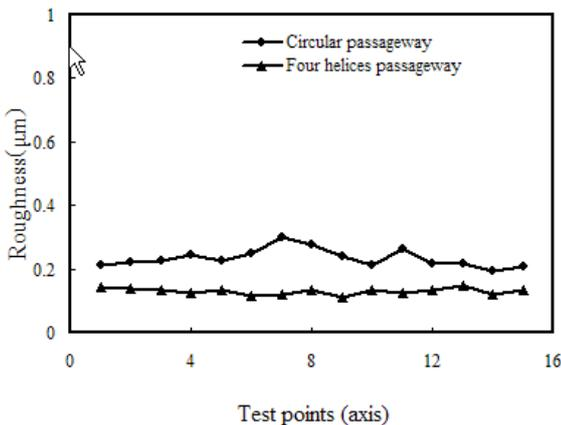
Fig. 8. The comparison curves diagram for helical passageway effects on uniformity of surface roughness.
