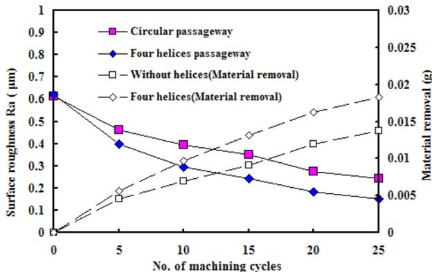
Fig. 7. The comparison curves diagram for helical passageway effects on surface roughness and material removal rate.
