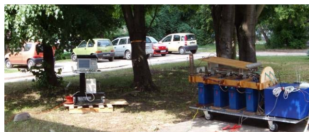
Fig. 2. Step voltage measurements in progress
