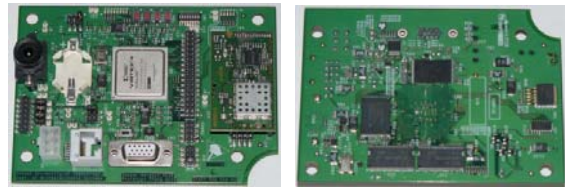
Fig. 4. The assembled main board of the system (FPGA prototype #2)
