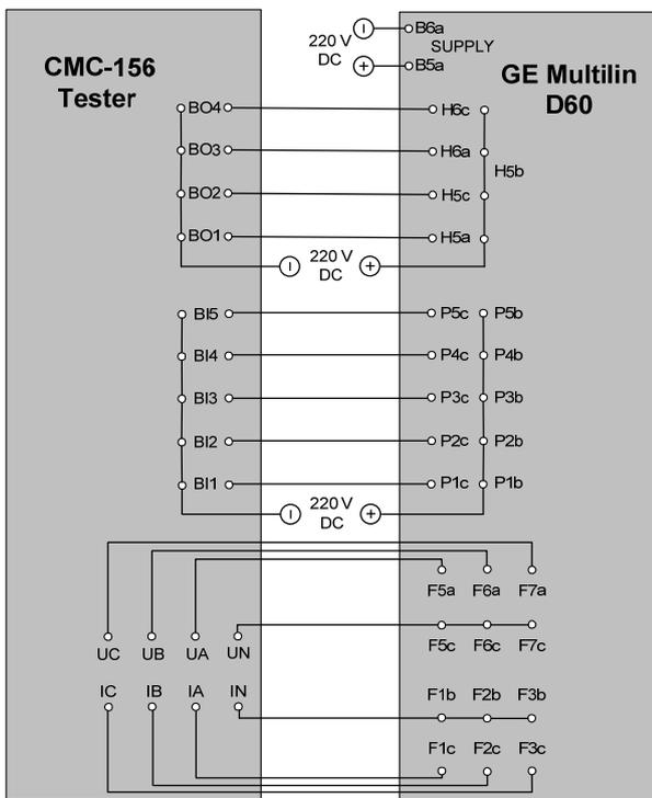
Fig. 1. Connection diagram of D60 and CMC-156 tester during synthetic tests of D60 pilot schemes functions
