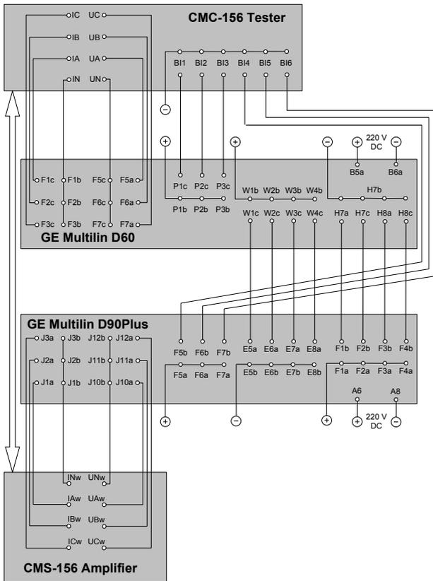
Fig. 4. Connection diagram of D60 and CMC-156 tester during synthetic tests of D60 pilot schemes functions
