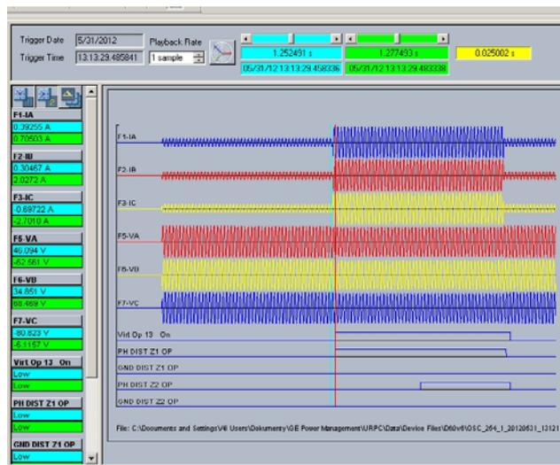
Fig. 3. Internal D60 device oscillography record for symmetrical fault
