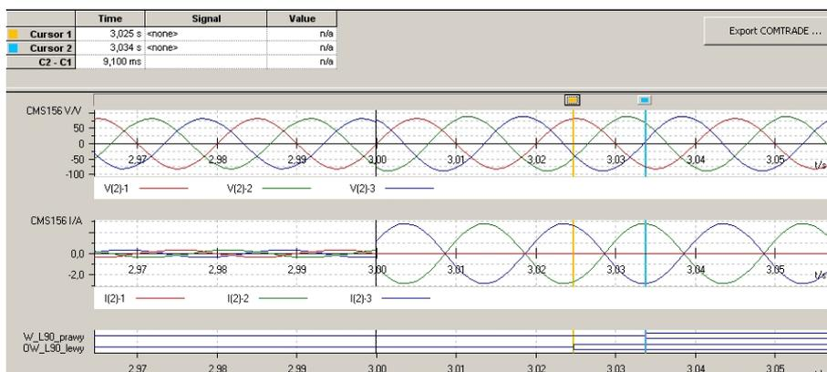
Fig. 8. Example of tripping delay measurement for phase-to-phase fault near L90 (2) device (called “L90\_lewy”)
