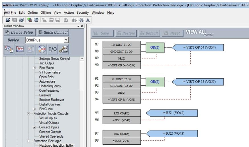
Fig. 6. Screenshot of *EnerVista UR Plus Setup* software window: functions tree on the left; on the right – visualisation of programmable logic (*Flex Logic*) settings
