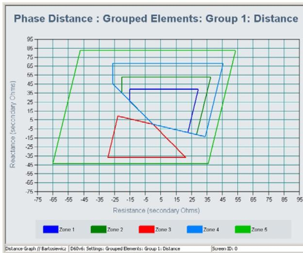
Fig. 2. Distance graph for example D60 phase-distance function settings
