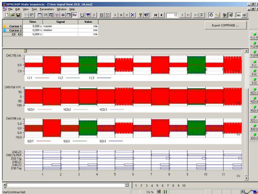
Fig. 7. Test results of DCB pilot scheme (with 4-bit signal coding) for six types of faults (simulated on even seconds): first three internal faults and second three external faults (accordingly symmetrical, phase-to-phase and phase to ground fault for each fault location); Z1, Z2, Z4 – zones 1, 2, 4; PKP – pick-up of relay in given zone; Trip – overall (measured) device trip
