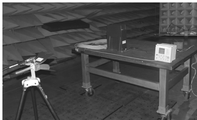
Fig.7. Electromagnetic field immunity test
