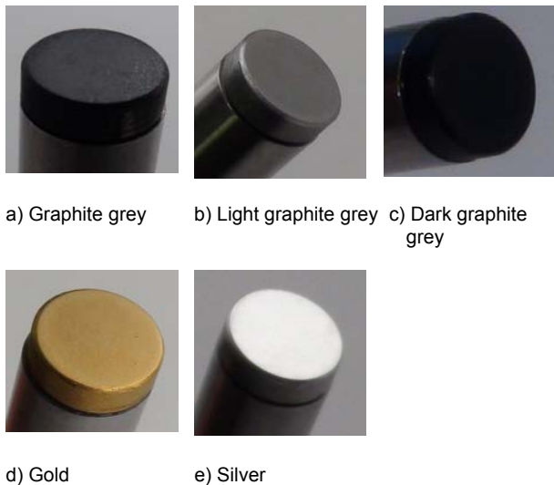
Fig.2. Test samples: a) aluminium, chromium and titanium nitride Al_{0,7}Cr_{0,15}Ti_{0,15}N , b) chromium nitride CrN, c) diamond-like surface a-C:H:N, d) titanium nitride TiN, e) aluminium Al
