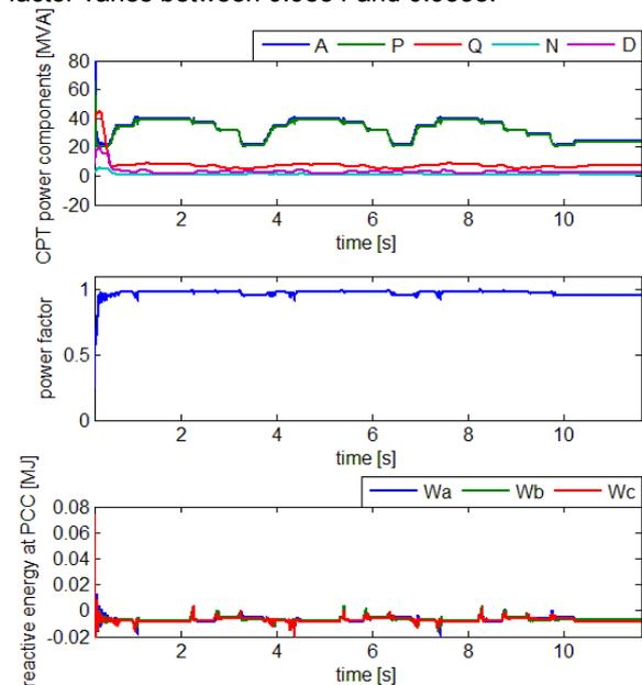
Fig. 5. CPT power components, power factor and reactive energies at PCC without compensators.
