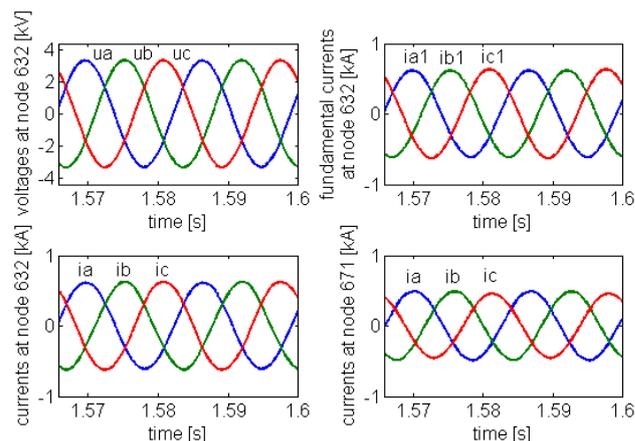
Fig. 11. Voltages (top left) and currents (bottom left) at PCC (node 632), fundamental currents (top right) from PCC and currents from node 671 (bottom right) after compensation.
