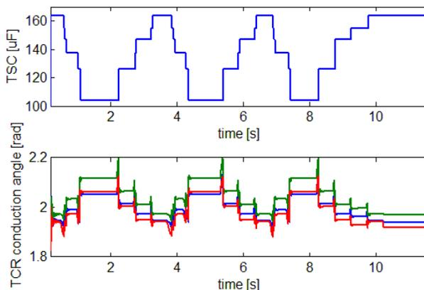
Fig. 7. TSC values (top) and TCR conduction angles (bottom).
