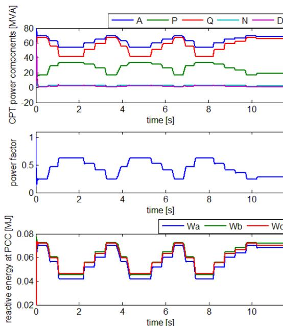
Fig. 4. CPT power components, power factor and reactive energies at PCC without compensators.
