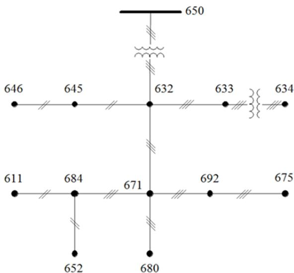
Fig. 9. IEEE 13 node test feeder-based network [17].
