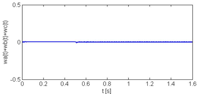
Fig. 12. Sum of instantaneous reactive energies from node 632 at each instant of simulation.
