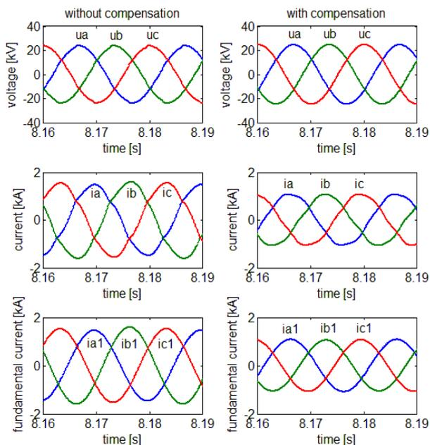
Fig. 6. Voltages (top), total currents (center) and fundamental component of the currents (bottom) at PCC with (left) and without (right) compensation.
