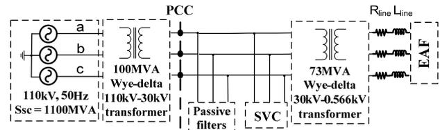
Fig. 3. Topology of the compensators for local compensation. Equivalent line impedance:  $R_{line} = 0,478m\Omega$ ;  $L_{line} = 10,66\mu H$ .
