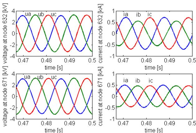
Fig. 10. Voltages (left) and currents (right) at PCC (node 632) and node 671 without compensation.
