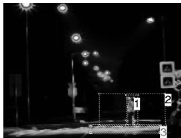
Fig 2: Luminance analysis of pedestrian crossing – luminaire MACH1
