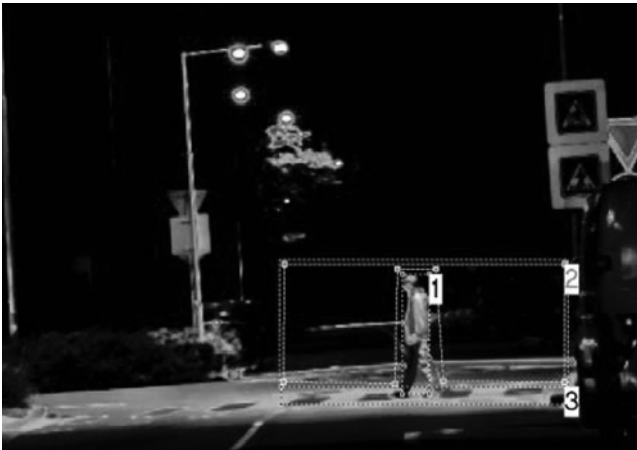
Fig 4: Luminance analysis of pedestrian crossing – luminaire Areaflood
