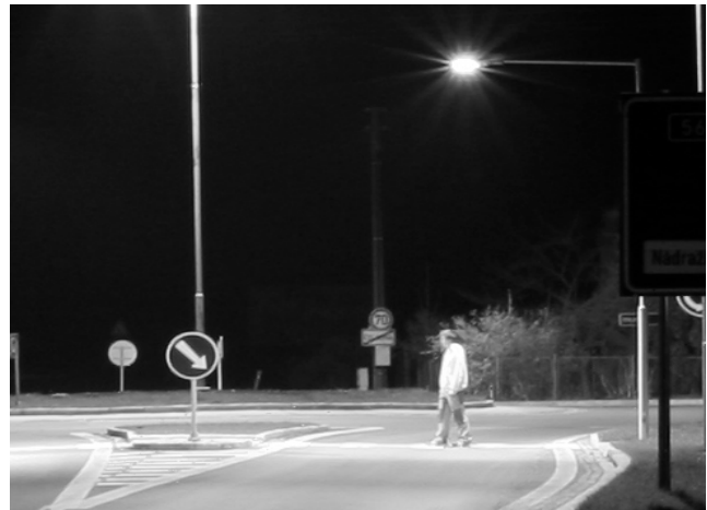
Fig 5: Photography of pedestrian crossing – metal halide lamp
