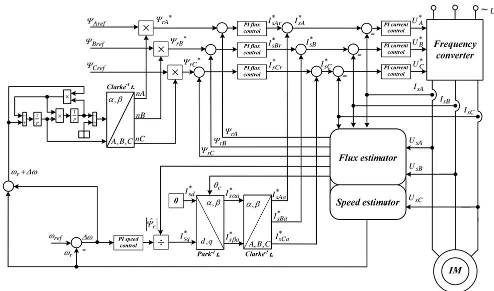
Fig.3 Block diagram of sensorless VCS with separate regulation of phases flux linkages
