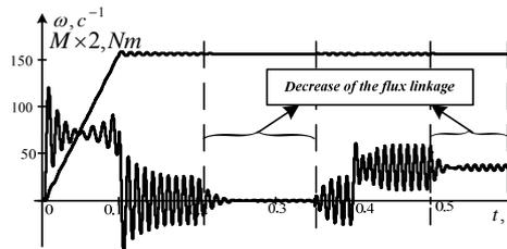
Fig. 6 Speed and moment transient processes in ED with VCS and IM stator winding asymmetry with and without compensation
