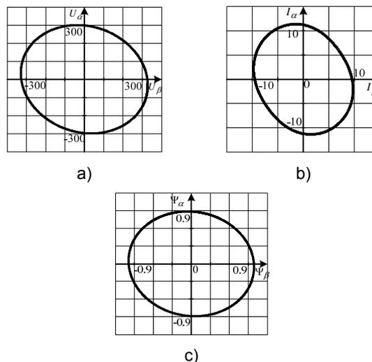
Fig. 5 Hodographs of IM voltage (a), current (b) and rotor flux linkage (c) in the system of separate vector control with asymmetric stator windings (windings asymmetry coefficient is 10%) with windings asymmetry compensation by decrease of asymmetric phase flux linkage by 10%
