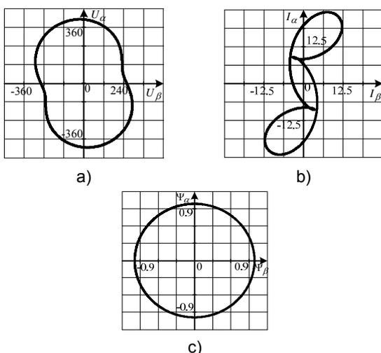
Fig. 4 Hodographs of IM voltage (a), current (b) and rotor flux linkage (c) in the system of separate vector control with asymmetric stator windings (windings asymmetry coefficient is 10%) without windings asymmetry compensation
