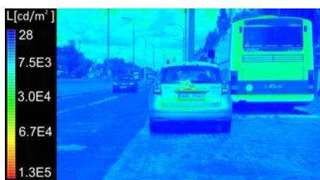
Fig. 3 Environment luminance distribution [cd/m 2 ]. daytime, summer, vehicle directly illuminated by the sun.
