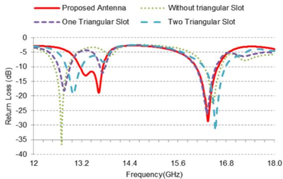
Fig. 3. Simulated S<sub>11</sub> of the four types of antenna
