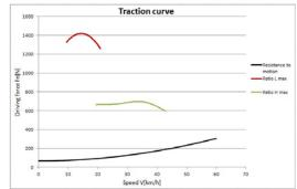
Fig.5. UTV vehicle traction curve - combustion engine
