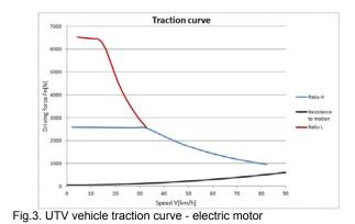
Traction curve (Fig. 4) presents the course of acceleration of the vehicle at different transmission ratios (High and Low) as vehicle speed function at full engine power. Calculations were made on the basis of table 4.
