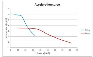
Fig.4. UTV vehicle acceleration curve - electric motor
