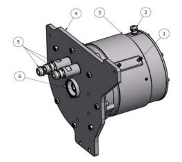
Fig.2. Conceptual model of electric engine with permanent magnets 1 - water jacket, 2 - enkoder cable gland, 3 - machine body, 4 assembly plate, 5 - power supply cable glands, 6 - seal sleeve
