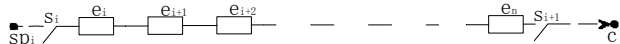
Fig.2. A typical radial feeder ( SP is power, S is switch, e is device, c is customer.).
