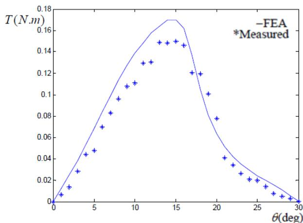
Fig. 4. Static torque rotor position for  $i=2.5$  A
