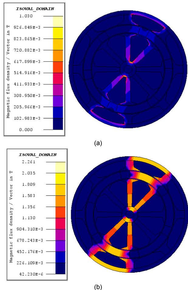
Fig. 2. Flux density distribution of the DSSRM A) unaligned b) aligned
