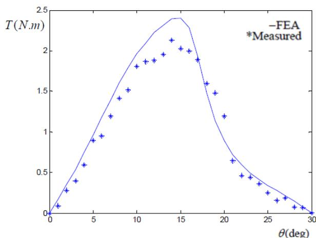
Fig. 5. Static torque rotor position for  $i=10$  A
