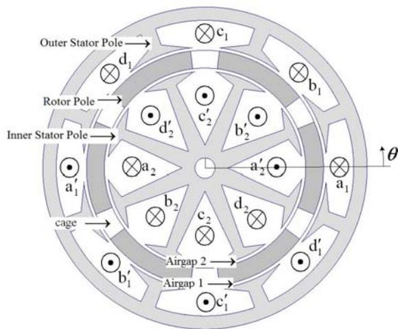
Fig. 1. Cross section of a 8/6 four-pole DSSRM
