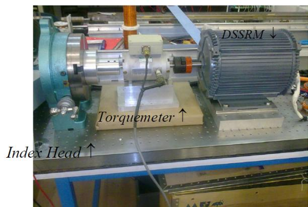
Fig. 3. The test set-up for the static torque measurement.
