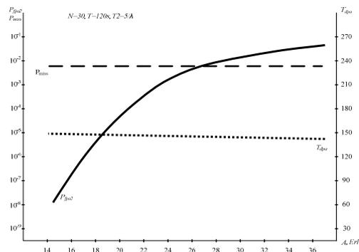
Fig. 7. Probability of false pre-alarm, probability of miss and mean time to detection of two-step detector as functions of offered traffic
