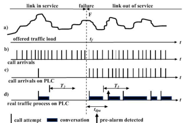
Fig. 5. Symbolic presentation of traffic process and two-step detector activation: a) (hypothetical) offered load, b) total call arrivals, c) call arrivals to PLC, d) detector activation
