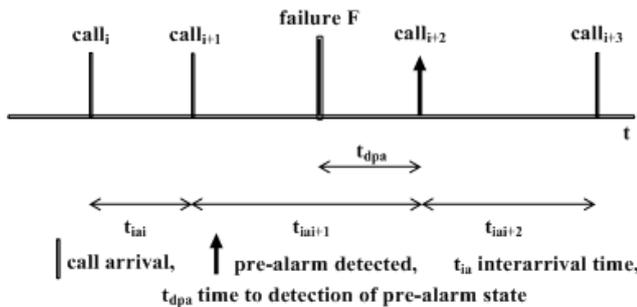
Fig. 3. Presentation of activation of one-step detector
