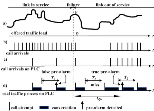
Fig. 6. Symbolic presentation of: a) (hypothetical) offered load, b) total call arrivals, c) call arrivals to PLC, d) false pre-alarm, miss and true pre-alarm (two-step detector)
