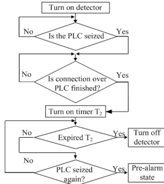
Fig. 4. Flow-chart of two-step detector operation
