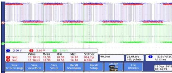
Fig.14 Generated two complementary pulses with frequency\_ref=10.5Hz
