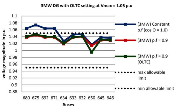
Fig. 4: Voltage magnitude at different buses with 3 MW of DG operating at constant power factor set at (i) 1.0 p.f., (ii) 0.90 p.f., and (iii) 0.90 p.f., with OLTC set at  $V_{max} = 1.05$  p.u.
