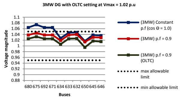
Fig. 5: Voltage magnitude at different buses with 3 MW DG operating at constant power factor set at (i) 1.0 p.f., (ii) 0.90 p.f., and (iii) 0.90 p.f., with OLTC set at  $V_{max} = 1.02$  p.u.
