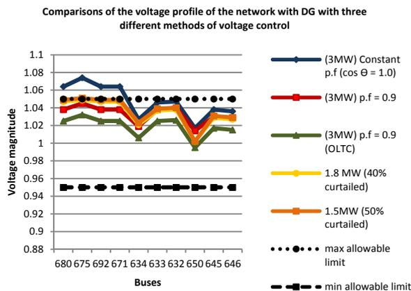
Fig. 7: Comparison of the effectiveness of the three different voltage control methods in managing voltage rise issues in an IEEE 13 bus network with DG.
