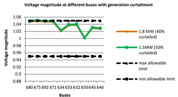
Fig. 6: Voltage magnitude at different buses with generation curtailment option.
