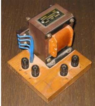
Fig.6. The tested single phase transformer
