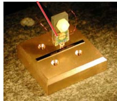
Fig. 9. Sample of microscope BEMI head mounting solution
