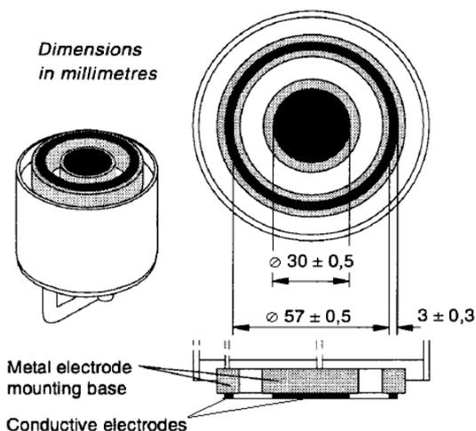
Fig. 8. Surface resistance measurement electrode assembly [7]
