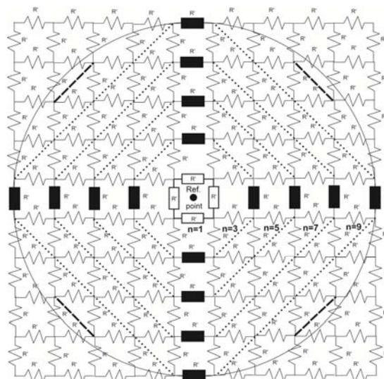
Fig. 9. Modelling of circle segment of grid of resistors
