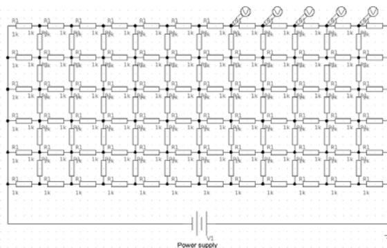
Fig. 3. Voltage probes placed in the points with different potential
