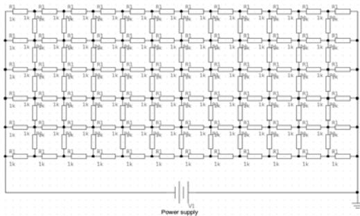
Fig. 1. Equivalent circuit diagram of used textile material
