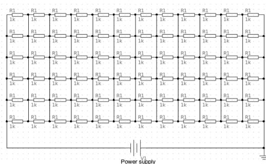
Fig. 2. Simplified equivalent electrical circuit with eliminated resistors placed between two points of the same potential
