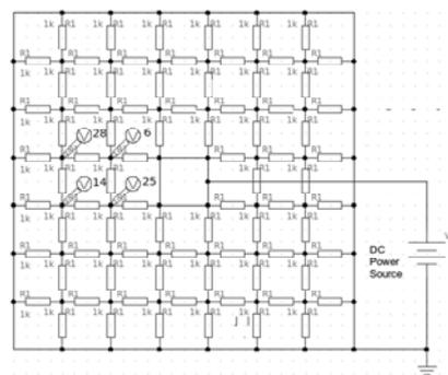
Fig. 10. Modelling of circle segment of grid of resistors
