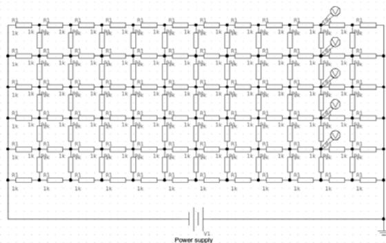
Fig. 5. Voltage probes placed in the points with the same potential
