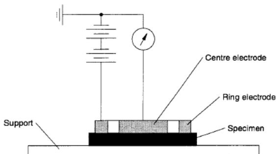
Fig. 7. Surface resistance measurement connection [7]
