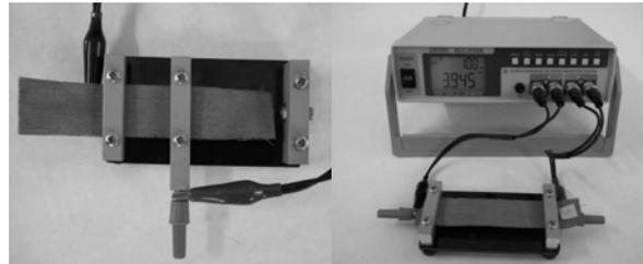
Fig. 16. Resistance measurement diagram (left) and square setting of electrodes (right)
