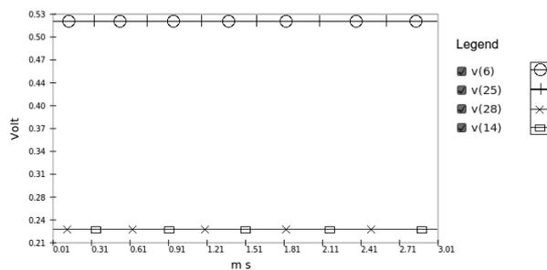
Fig. 11. Measurement results of voltage probes for nodes with same potential levels (v6 and v25) and (v14 and v28)
