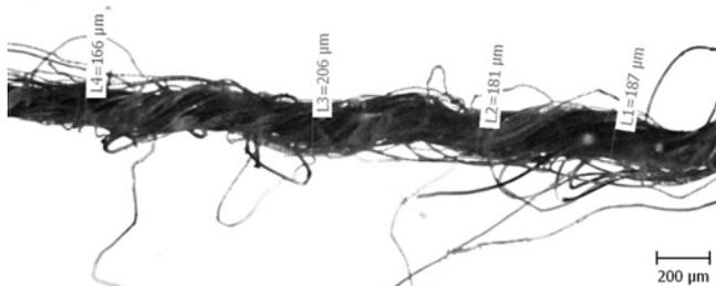
Fig. 15. Diameter measurement places of fibre from sample No. 60
