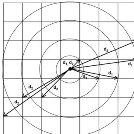
Fig. 13. Circle diameter  $d_1$  and square diagonals  $d_2$  determination
