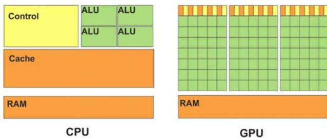
Fig.1 CPU and GPU architecture
