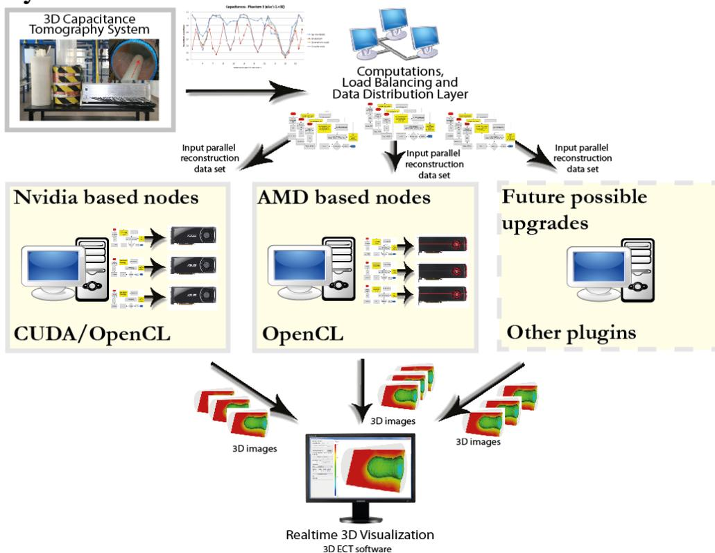
Fig. 2. Distributed computational system for accelerating image reconstruction in Electrical Capacitance Tomography
