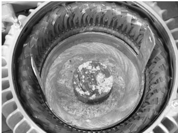
Fig.2. Working version of the device for platinum leaching from used auto catalytic converters
