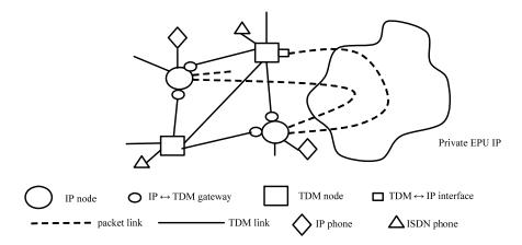
Fig.1. Symbolic presentation of the mixed EPU telephone network
