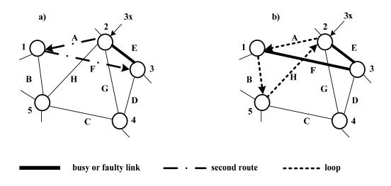
Fig.3. Call routing in the case of busy or faulty links
