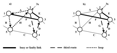
Fig.4. An example how to avoid forming an indefinite loop
