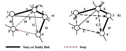
Fig.5. An example how to avoid forming the loop if in some node the link of last choice is not used
