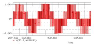
Fig.4 Exemplary runs of phase voltage with a 3-phase supply of load of type RL by a voltage inverter with PWM modulation
