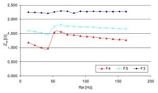
Fig. 11 Results of determination of input impedance module of one drive group for three versions of an input filter F4 ( $L_f$  = 8,7 mH,  $C_f$  = 2 mF); F5 ( $L_f$  = 8,7 mH,  $C_f$  = 2,8 mF); F3 ( $L_f$  = 8,7 mH;  $C_f$  = 6,5 mF)
