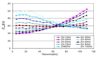
Fig. 8 Module of input impedance of a drive system in the function of inverter frequency  $f_{fal,,}$  for selected frequencies with constant depth of modulation  $M_{mod}{=}0,6$
