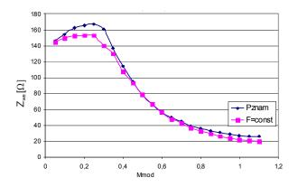
Fig. 9 Module of input impedance of a drive system in the function of modulation depth for the frequency of 50 Hz, where:  $P_{znam}$  -frequency of an inverter that changes fluently together with modulation depth  $F_{const}$  - constant inverter frequency
