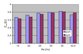
Fig. 6 Comparison of the results of impedance module determination by computer simulation (sym) with the results of laboratory measurements (pom) for various frequencies of converter operation ( $f_{ral}$ ) ith inductance of input filter L<sub>F1</sub> = 1,8mH a) impedance for harmonic 41 Hz b) impedance for harmonics 46 Hz
