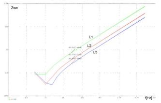
Fig. 14 Exemplary run of module of input impedance of vehicle input filter for different inductance values :L1=24mH, L2=12mH L3=8mH
