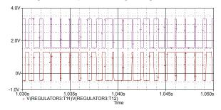
Fig. 3 Exemplary runs of the signals controlling the "upper" and "lower" key of an individual inverter branch
