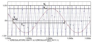
Fig. 2 Runs of signals compared to the generation of runs which control inverter branches, where:  $V_{sin^-}$  an amplitude of sinusoidal signal,  $V_{tr}$  – an amplitude of triangular signal,  $T_{sin}$  - a period of sinusoidal signal,  $T_{tr}$  – a period of triangular signal
