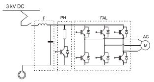
Fig. 5 Exemplary scheme of main circuit for one driving group of a vehicle powered by asynchronous motors supplied by voltage inverter AC/DC.
