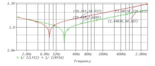
Fig. 12. Characteristics of impedance module of exemplary input filters allowing for the fulfilment of the norm PN-EN 50388 [13] for multiple-operation of a 4-motor vehicle with accordance to the a) effective version (1/I(Lf15)  $L_f$  = 10mH), b) previous version (1/I(Lf16)  $L_f$  = 60mH)
