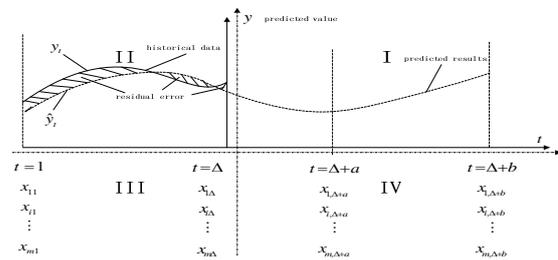
Fig.4. Prediction principle diagram of semi-parametric model with multiple impact factors
