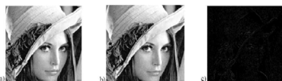
Fig.2. Image a) original image, b) shifted, c) the difference between original and shifted images
