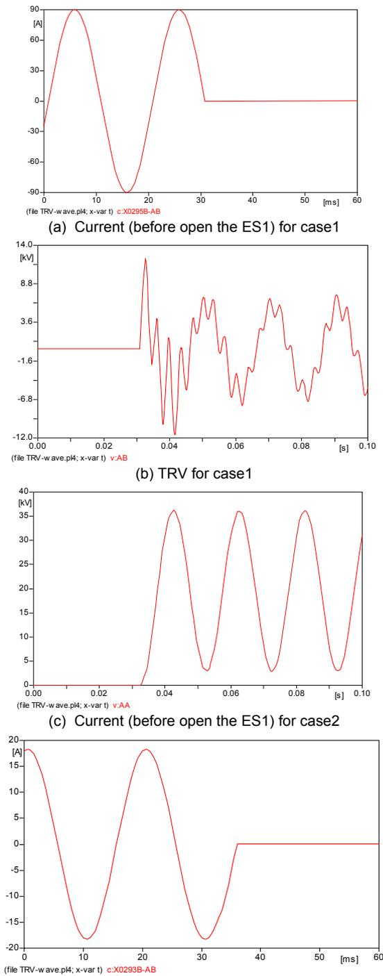
Fig.7 The current and TRV for case1 and case2
