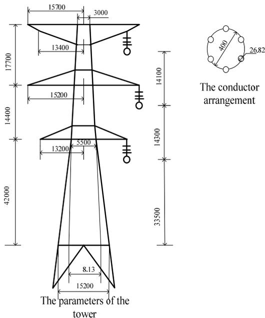
Fig. 5. Arrangement of the conductors of a 750kV double-circuit lines on the same tower
