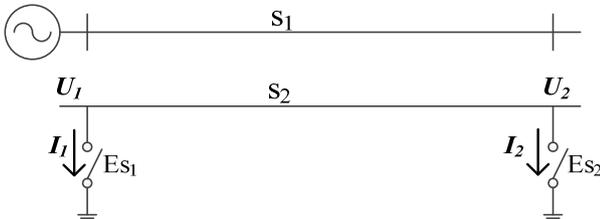
Fig. 2. Both ends of the maintenance lines are opened
