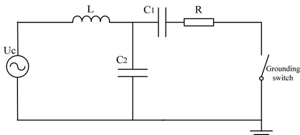
Fig.9 Test circuit for capacitive switching  $U_S=100kV$   $C_1=3.73\mu F$   $C_2=3.19\mu F$   $R=38\Omega$
