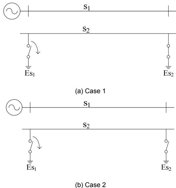
Fig.6 Two cases of the grounding switches operation
