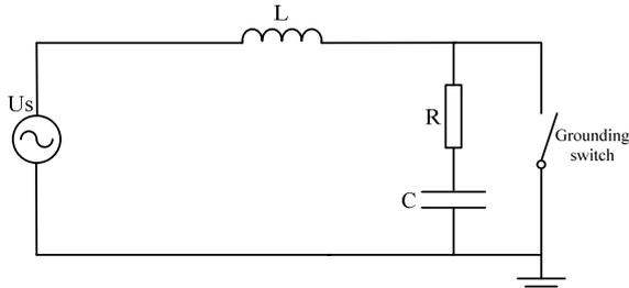
Fig.8 Test circuit for inductive switching  $U_S=39kV$   $X_L=65\Omega$   $C=6\mu F$   $R=38\Omega$
