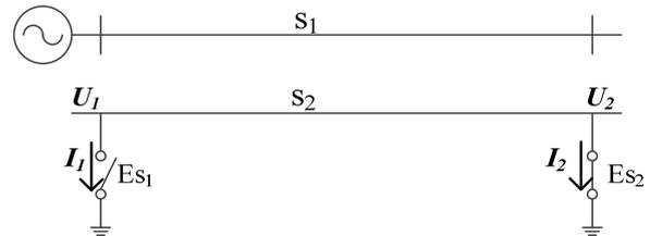
Fig. 3. The sending end is opened and the receiving end is closed
