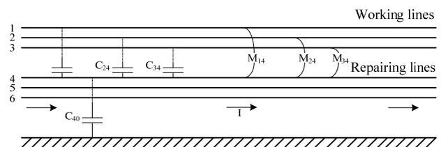
Fig. 1. The calculation model of the coupling effects between the double circuits transmission line
